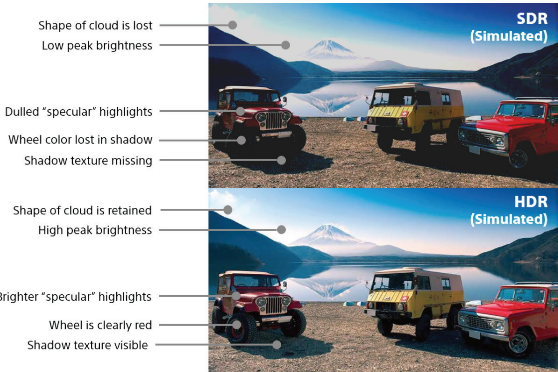
This pair of simulated images illustrates how SDR clips highlight details and crushes black details that HDR retains.
